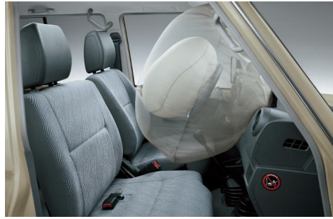
Front-seat dual SRS* airbags supplement the restraining action of seatbelts to provide further protection in the even of a front-end collision (Optional)
