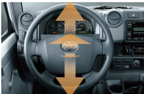
A tilt-adjustable, telescoping steering wheel allows finer adjustments to maximise driving comfort
