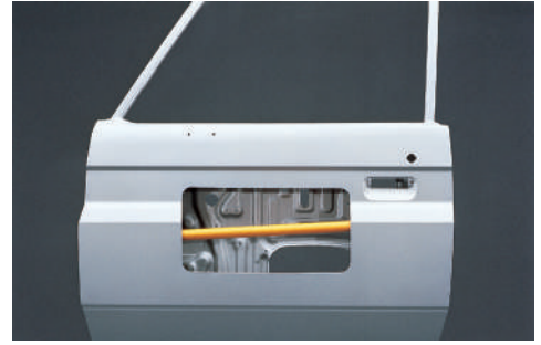
Side impact beams reduce the likelihood of side impact intruding through the doors
